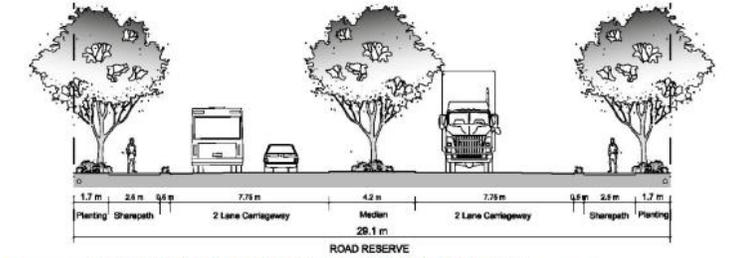
4 Lane Sub-Arterial Road with off road cycle / shared path (source: DCP)
