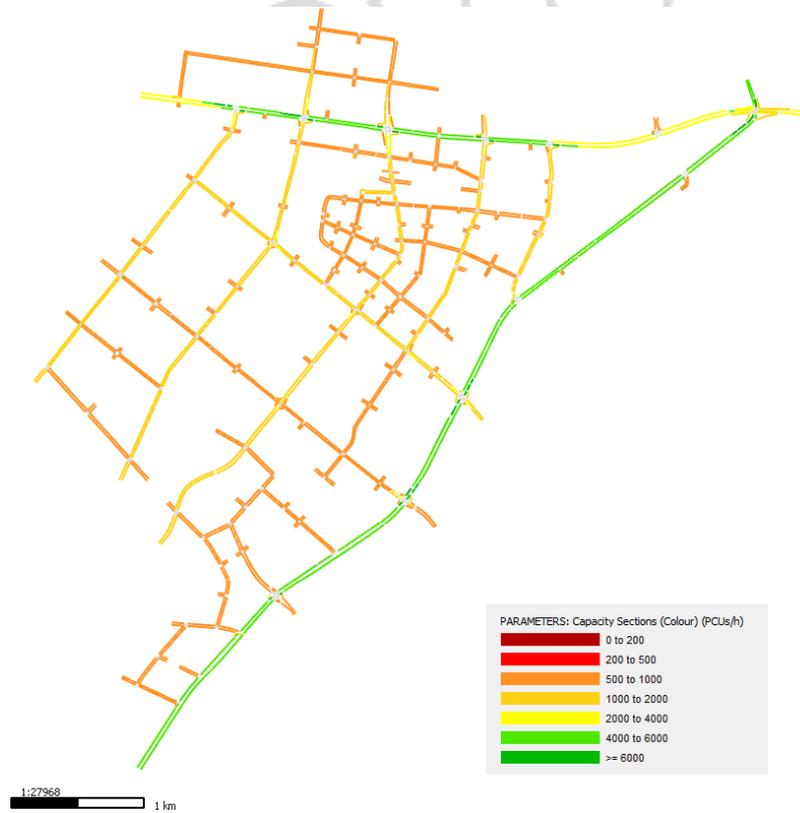
Figure 9: Roadway capacity for future roads (per direction)
